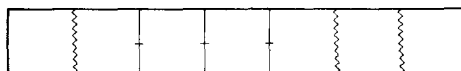
FIG. 4. The seven vacancies shown in Fig. 3 have N - q - 1 = 6 partitions between them. n_{00} = 3 of these partitions separate vacant nearest neighbor pairs (short horizontal lines) and three do not (jagged lines). There are \binom{6}{3} = 20 ways of arranging the separating partitions to form the N - q - n_{00} = 4 “units” illustrated in Fig. 3.
